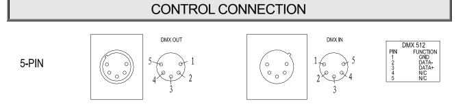
Connection between the controller and a projector and between one projector and another must be made with a 2 core-screened cable, with each core having at least a 0.5mm diameter. Connection to and from the projector is via
