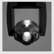
The VARI\*LITE<sub>®</sub> VL6C<sup>™</sup> spot luminaire is an improved version of the VL6B<sup>™</sup> luminaire and features a 700 watt short arc lamp and a new cold mirror reflector to provide an extremely bright and flat field. The luminaire is small, lightweight and virtually silent.
