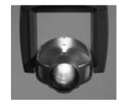
The VARI\*LITE® VL6B™ spot luminaire adds a zoom optics system and rotating gobos to the VL6™ feature set. It uses the Philips MSR 400W short arc lamp in a cold mirror reflector. The luminaire is small, lightweight, and virtually silent.
