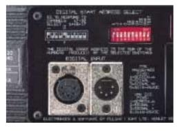
The inputs are protected against accidental injection of mains voltage, while a self-diagnostic routine makes it possible identify faults fast.
