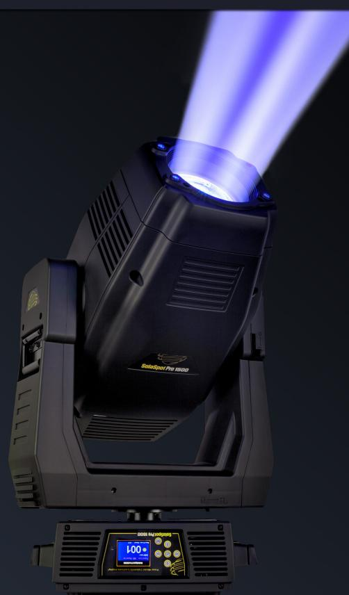
SolaSpot Pro 1500, the latest in the SolaSpot range, is an innovative and ground breaking fixture. The SolaSpot Pro 1500 outputs 20,000 lumens using a 400w LED engine! Unparalleled LED brightness coupled with features including framing shutters, CMY color mixing, linear CTO, two gobo wheels, animation effects, a prism, an iris, frost and an 8 to 45 degree zoom range (amongst others) make this the most exciting LED product on the market today.
