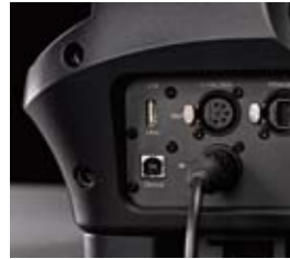
Included is a USB host socket that can be used to download the event log, upload firmware, and add prospective features.
