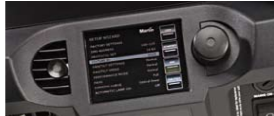
A unique LCD screen Graphical User Interface with jog wheel makes the MAC III Profile quick to program and troubleshoot - and easy to use. The LCD screen is battery-powered so that fixture status can be read while still in the flightcase.
