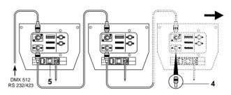
Projectors are wired up to the controller and one to the next using two-core screened cable and Cannon 5 pin XLR type plug/socket connectors.
