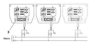
The projector is designed to operate at the voltage and frequency indicated on the electrical data plate (3) affixed to the rear end. Check that these two values correspond to the mains voltage and frequency.
