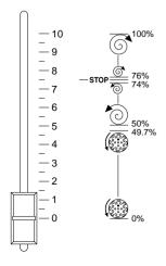
From 0% to 49.7% the internal dome turns anti-clockwise through 360°. When the slider reaches 50% the dome starts spinning at maximum speed and then it gradually slows down until it comes to a stop on 74%. At 76% the dome starts turning in the opposite direction starting from minimum speed and gradually accelerating up to maximum speed when the slider is on the 100% position.
