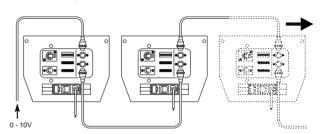
The connection between controller and projector must be made using a multi-core cable with 8 wires of 0.25mm² section and a DIN 8 PIN 45° plug/socket connector.
