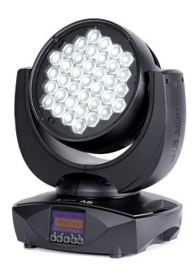
A8 Tunable White. The power-pack A8 is now also available with white LEDs. It is equipped with 37 multi-chip LEDs in the 15W class. Each multi-chip LED has two cold-white and two warm-white chips, which allow continuous adjustment of the colour temperature from 2900 Kelvin to 7700 Kelvin.
